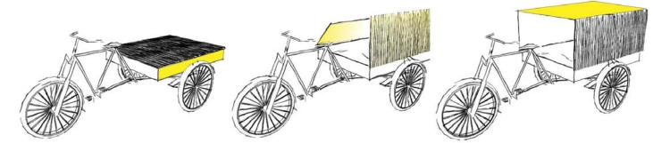
a. add small storage area under the van's bed where the van puller can store necessary belongings.
